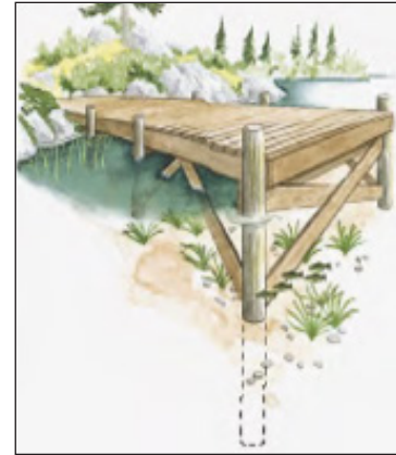
Figure 8: Permanent Post Dock
