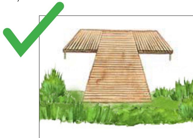
Figure 3: Dock oriented away from shore
